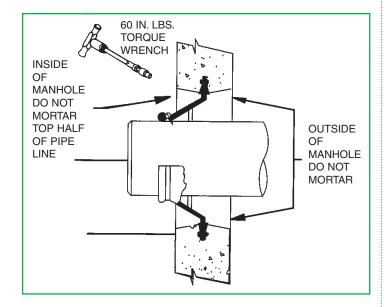
WARNING: To ensure the Z-LOK Connector remains a flexible watertight connector, it is A•LOK Products, Inc. strong recommendation that **no mortar** be placed between the pipe and wall of the concrete structure. The use of mortar in this area would decrease the effectiveness of the connector to compensate for shear caused by settlement or ground movement.
